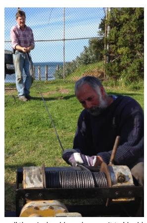
outa Boaters Ian and Gerrard took the chance to 'end for end' the winch cable and grease it to 'double' its life. Ant Grage installed the winch a few decades ago and after fairly minor repairs hopefully it will go for a a few more! The wiring was also 'fixed' again so In goes in and Out goes out.
